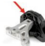
Engine Mount Technyl® A218V50 Bk 21N Polyamide 6.6 compound (50% glass fiber)
