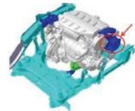
Engine Mount Technyl® A218V50 Bk 21N Polyamide 6.6 compound (50% glass fiber)
